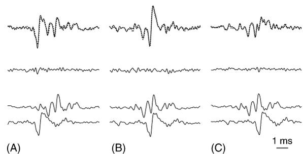
Fig. 3. Three very different looking superimpositions from the same two MUs. (A) Partial superimposition. (B) Constructive interference. (C) Destructive interference. Each set shows the superimposition (top solid), templates (bottom), reconstruction (top dotted), and residual (middle). All the signals have been interpolated to an effective sampling rate of 100 kHz.
