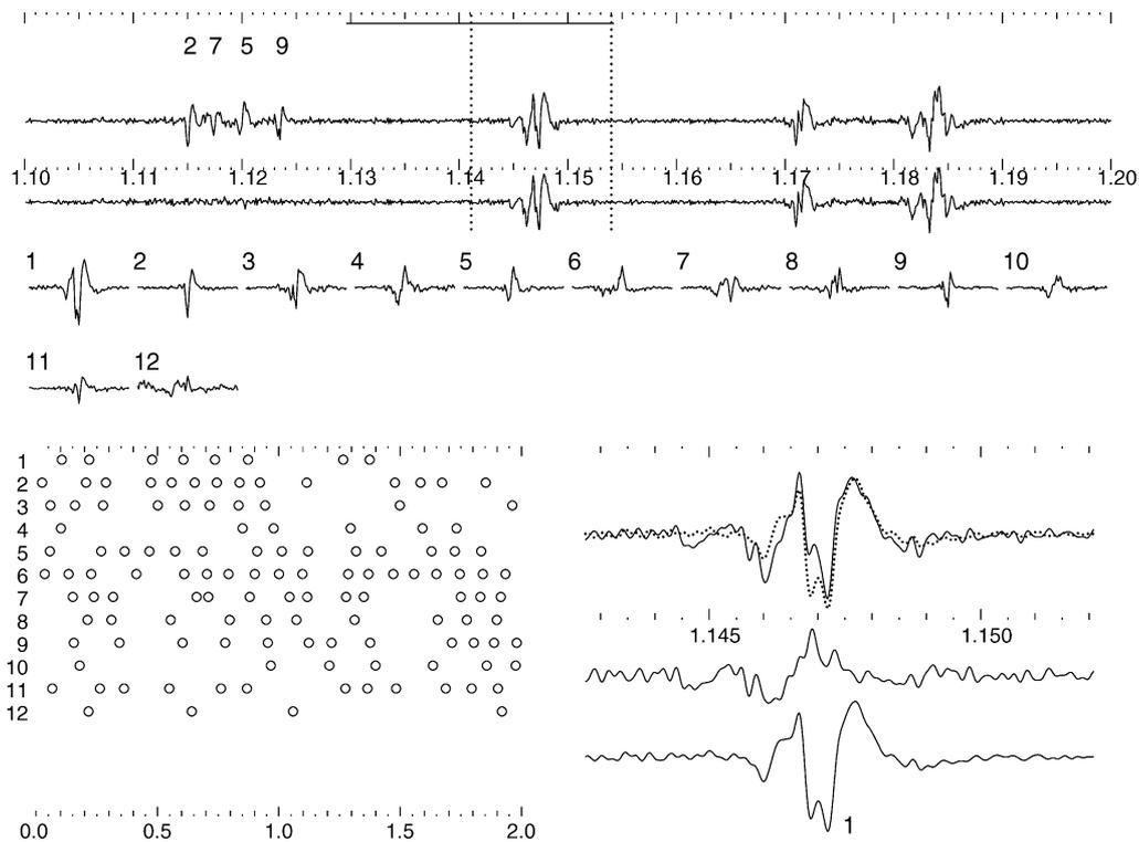
Fig. 5. EMGLAB screen after the initial automatic decomposition procedure for the signal of Fig. 1. The decomposition is incomplete and needs to be completed manually. The horizontal line in the signal panel shows the expected discharge time of MU 1. In the close-up panel, the template of MU 1 has been aligned with the spike at 1.148 s. The residual can be recognized as an occurrence of MU 4.
