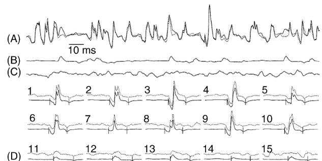
Fig. 8. MUP waveform averaging. (A) Unfiltered EMG signal from the semitendinosus muscle (solid) and reconstructed contribution of the 10 MUs that were decomposable in the signal (dotted). (B) Reconstructed contribution of five additional MUs decomposed from a nearby site. (C) Residual signal. (D) MUP waveforms obtained using averaging with (solid) and without (dotted) interference cancellation. The ticks indicate the MUP onsets and terminal waves.
